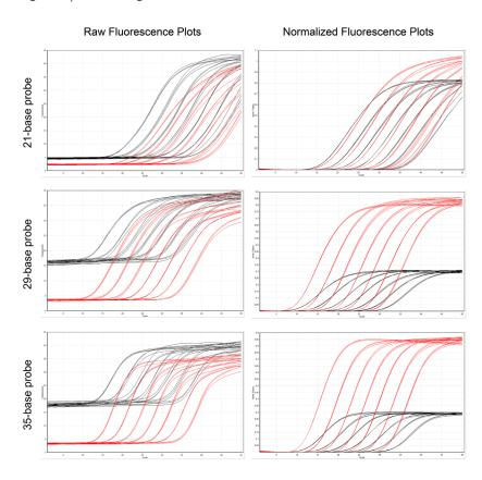
Figure 2 (on left) - Comparison of standard probes and BHQnova probes. Amplification traces signaled with traditional end-labeled probes in Black. Amplification traces signaled with doublequenched BHQnova probes in Red. The panels at left present the raw data while the panels at right present the same data following baseline subtraction and normalization.
