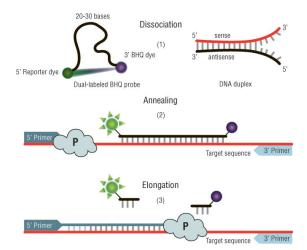
Fig. 1 – Signaling Mechanism of Hydrolysis Probes. After denaturation, the probe and primers anneal to the dissociated strands. During elongation the polymerase extends from the primer, encounters the probe, and hydrolyzes nucleotide fragments that then become displaced from the strand. Cleavage of the probe untethers the fluorophore and quencher to make signal release permanent.
